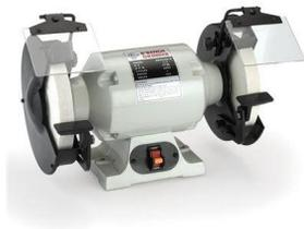
The Low Speed Bench Grinder is a machine used to drive an abrasive wheel or wheels. Depending on the grade of the grinding wheel, it may be used for shaping or sharpening the cutting edge of **lathe tools only**. To avoid accidents, the following operational safety rules must be observed by everyone working on the GWG Bench Grinder. **Failure to be certified or to follow the safety rules will result in loss of shop privileges.**
