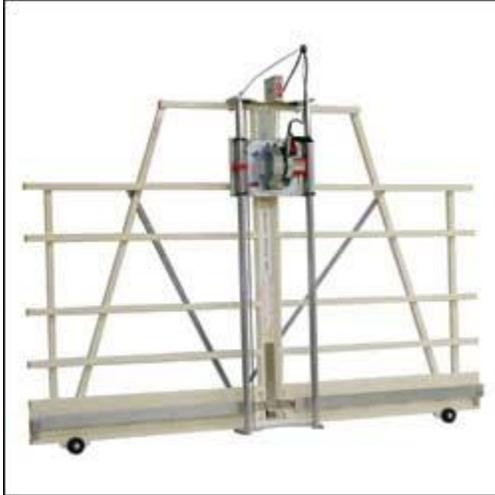
The Panel Saw is a specialized woodworking machine used to easily cut plywood, melamine, MDF or any sheet goods into cabinet components. To avoid accidents, the following operational safety rules must be observed by everyone working on the GWG Panel Saw. **Failure to be certified or to follow the safety rules will result in loss of shop privileges.**
