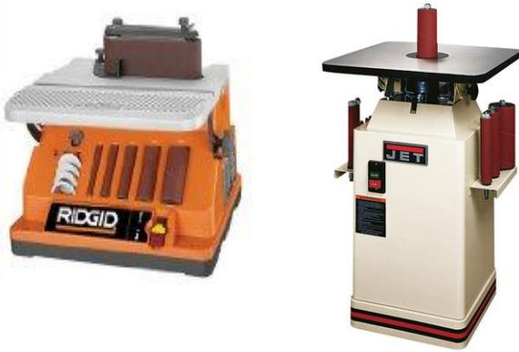
The Oscillating Spindle Sander is a sander mounted on a rotating spindle, but also moves up and down at the same time. Good for sanding curves and contours that would be difficult with hand sanding or orbital sanding. To avoid accidents, the following operational safety rules must be observed by everyone working on the GWG Spindle Sanders.
