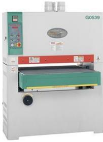
The Wide Belt Sander is similar to a thickness planer in that it removes material from the surface of a board. However, instead of using a series of knives and shaving the material, it uses a sandpaper belt to abrade the work piece that feeds through on a conveyer belt. To avoid accidents the following operational safety rules must be observed by everyone working on the GWG Wide Belt Sander. **Failure to be certified or to follow the safety rules will result in loss of shop privileges.**
