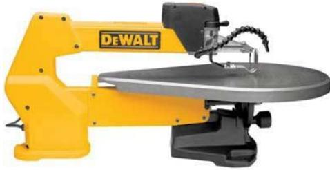
The Scroll Saw is used to make intricate cuts in wood up to  $\frac{3}{4}$  inches thick. The saw blade moves up and down and cuts on the down stroke. To avoid accidents, the following operational safety rules must be observed by everyone working on the GWG Scroll Saw. **Failure to be certified or to follow the safety rules will result in loss of shop privileges.**
