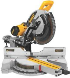
The Miter Saw is a power tool used to make quick, accurate crosscuts, miter or bevels. To avoid accidents the following operational safety rules must be observed by everyone working on the GWG Miter Saw. **Failure to be certified or to follow the safety rules will result in loss of shop privileges.**
