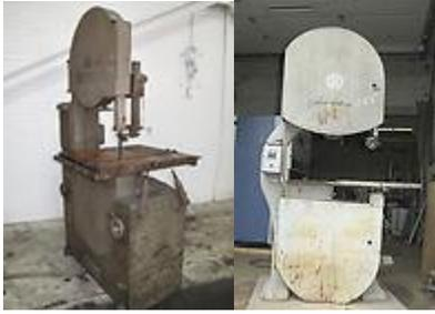
The 36” Band Saw has a thin vertical blade that allows cutting curves, re-sawing and large deep cuts on thick material. To avoid accidents the following operational safety rules must be observed by everyone working on the GWG 36” Band Saws. **Failure to be certified or to follow the safety rules will result in loss of shop privileges.**
