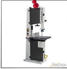
The 14 & 16” Band Saw has a thin vertical blade that allows cutting curves, re-sawing and large deep cuts on thick material. To avoid accidents the following operational safety rules must be observed by everyone working on the GWG Band Saw. **Failure to be certified or to follow the safety rules will result in loss of shop privileges.**
