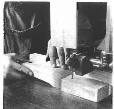
5. Saw out the leg post, and keep the sawn face as smooth as possible. You can use a table saw, but you'll have to finish the cuts with a handsaw or bandsaw. You can also remove the waste by making successive cuts on the radial-arm saw.
