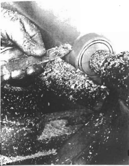
1. Center the bandsawn leg on the lathe, with the foot at the tailstock end, and turn the major diameter of the foot.
