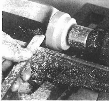
2. Mark the height of the foot pad on the cylinder, turn the pad to size and shape the sides of the foot to the correct profile. Scrape the pad with a parting tool—it's difficult to cut with a gouge or skew in such a small area. Make a shallow groove at the top of the foot with a skew to define the top edge when you carve the foot and the ankle. (You can also turn a small shoulder above the incised line, which rounds off the arris at the back of the ankle and causes the three other thin corners to flake off.) Shape the curved profile of the foot, and use the point of the skew to turn a crisp corner between the upper part of the foot and the pad. Finally, sand the foot on the lathe.
