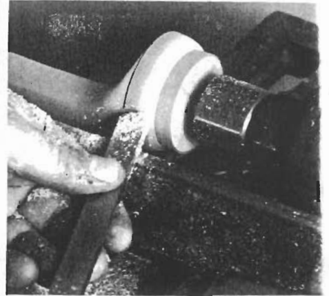
2. Mark the height of the foot pad on the cylinder, turn the pad to size and shape the sides of the foot to the correct profile. Scrape the pad with a parting tool—it's difficult to cut with a gouge or skew in such a small area. Make a shallow groove at the top of the foot with a skew to define the top edge when you carve the foot and the ankle. (You can also turn a small shoulder above the incised line, which rounds off the arris at the back of the ankle and causes the three other thin corners to flake off.) Shape the curved profile of the foot, and use the point of the skew to turn a crisp corner between the upper part of the foot and the pad. Finally, sand the foot on the lathe.
