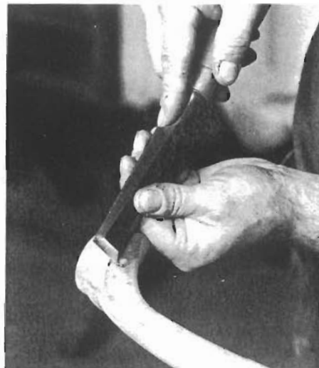
4. With a chisel, carve the ankle beyond the bandsawn line to give the foot more definition.
