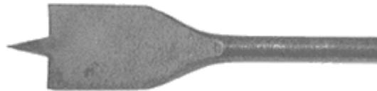
Intended for power drill use only, the centre point locates the bit and the flat steel on either side cuts away the timber. These bits are used to drill fairly large holes and they give a flat bottomed hole (with a central point) so are ideal where the head of a screw/bolt needs to be recessed into the timber - always use this bit before drilling the clearance hole for the bolt.
